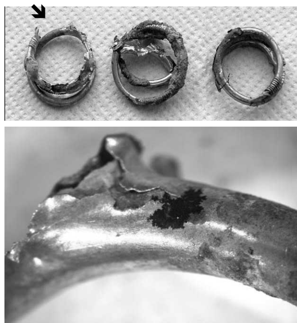
Figure 5 - Optical micrograph of gold plated brooches for braid of hair (top) with the enlargement of a cracked area of the artifact on the left (bottom).
