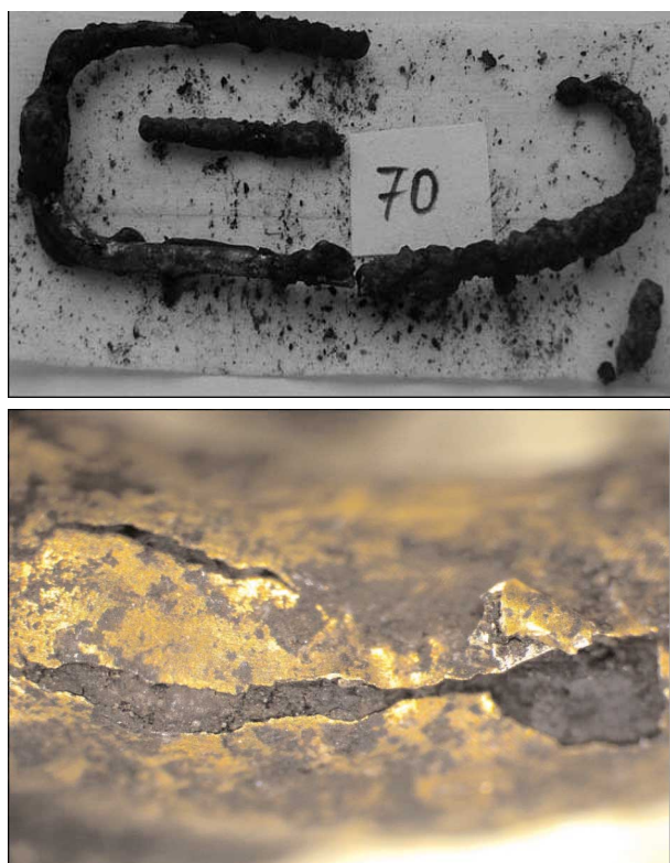
Figure 4 - Optical micrograph of a gold plated silver leech-shaped earring (top) with the enlargement of the cracked area (bottom).
