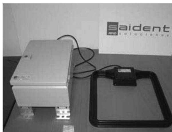
Figure 5: A RFID reader (left) and its antenna
